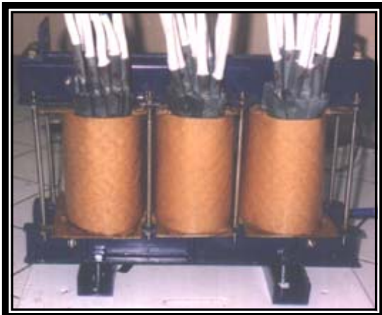
Oil Type Transformers with Tap Setting Assembly
