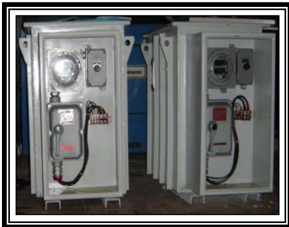
Oil Type Explosion Proof NEMA 4 CP Rectifier
